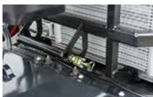
The front axle lubrication points are located in front of the radiator assembly for optimum accessibility.
