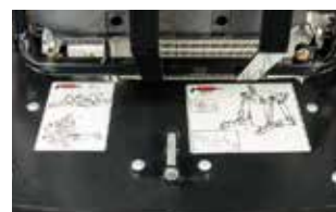
A lubrication chart under the hood simplifies maintenance.
