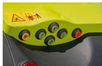
External controls for rear PTO on both fenders.
